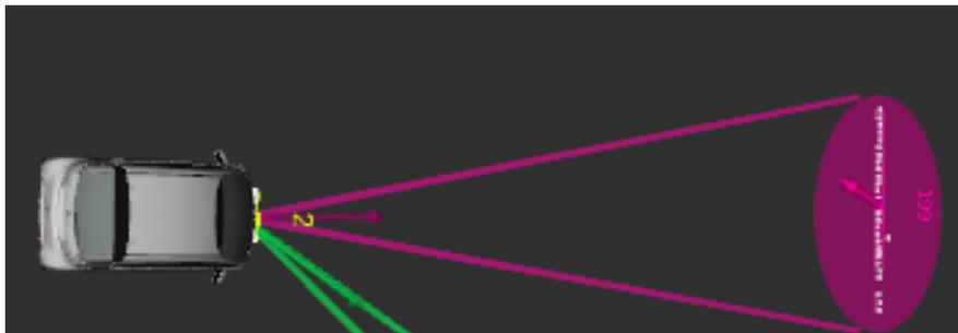
Figure 6.16: Rviz representation of the ATLASCAR2 sideways collision experiment with the target id 199. The collision cone can also be seen with the pink lines as well as the enlarged target circle.
