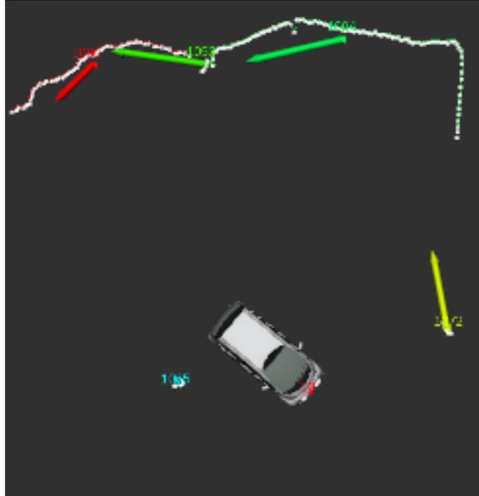
Figure 6.7: Rviz representation of the Rotating Around Two Pedestrians experiment error. The target placed in the turning center point is still being tracked with the same id 1065, however the target outside the turn (id number 1053) is being embraced by the background measurements, causing the target to merge with the remaining points and therefore lose the pedestrian tracking.
