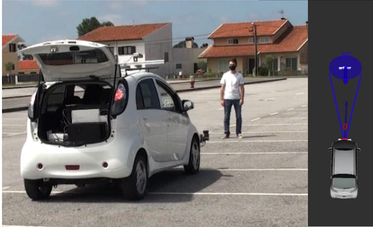
Figure 6.2: Front collision setup on the left and on the right the Rviz visualization of the VO cone (the blue lines) as well as the enlarged target circle .
